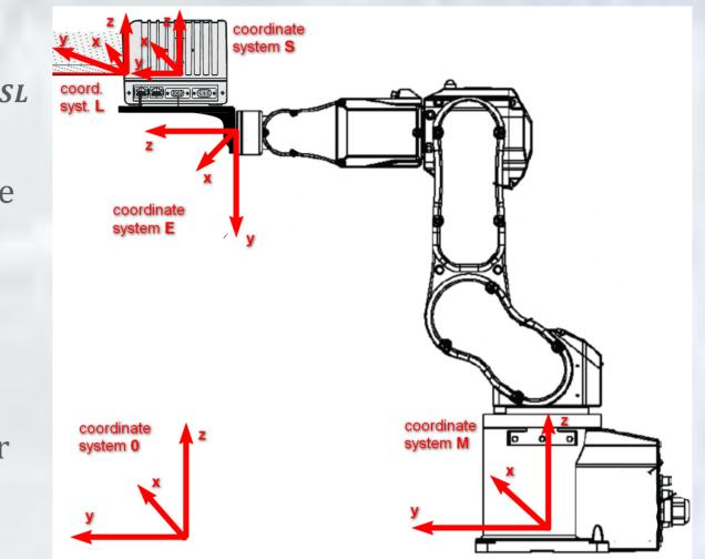
4. Calibration Procedure – uncommon solution: using generic calibration object instead of precise one + hybrid computing
