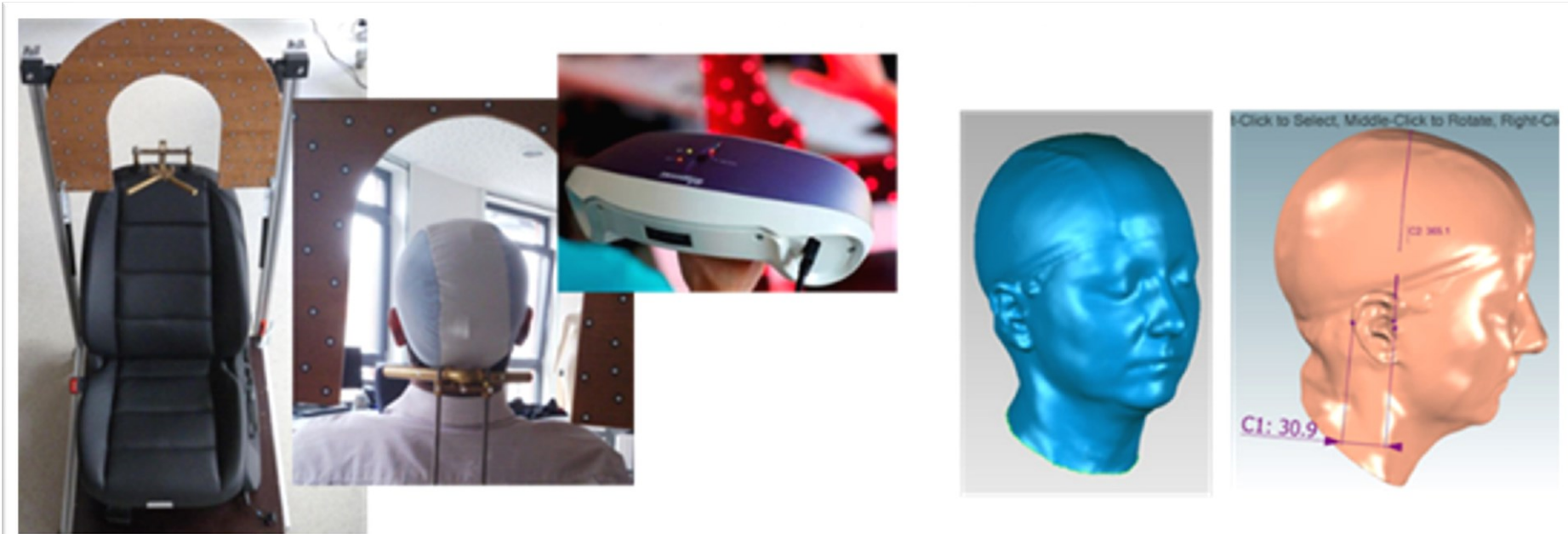
Fig. 3. 3D head scanning process with Creaform Erao Handvscan
